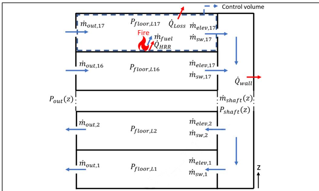
Figure 2. Reverse Stack Effect phenomenon. (Bilyaz et al., 2021)
