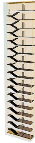
The position of the fire source and the opening of the stairwell model in PyroSim
