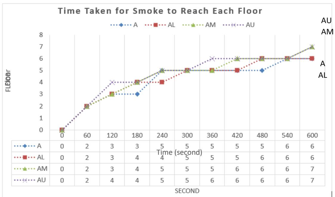
**Figure 5.** Time Taken for Smoke to Reach Each Floor in Case A, AL, AM, and AU
