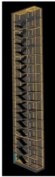
Stairwell model with walls in PyroSim
