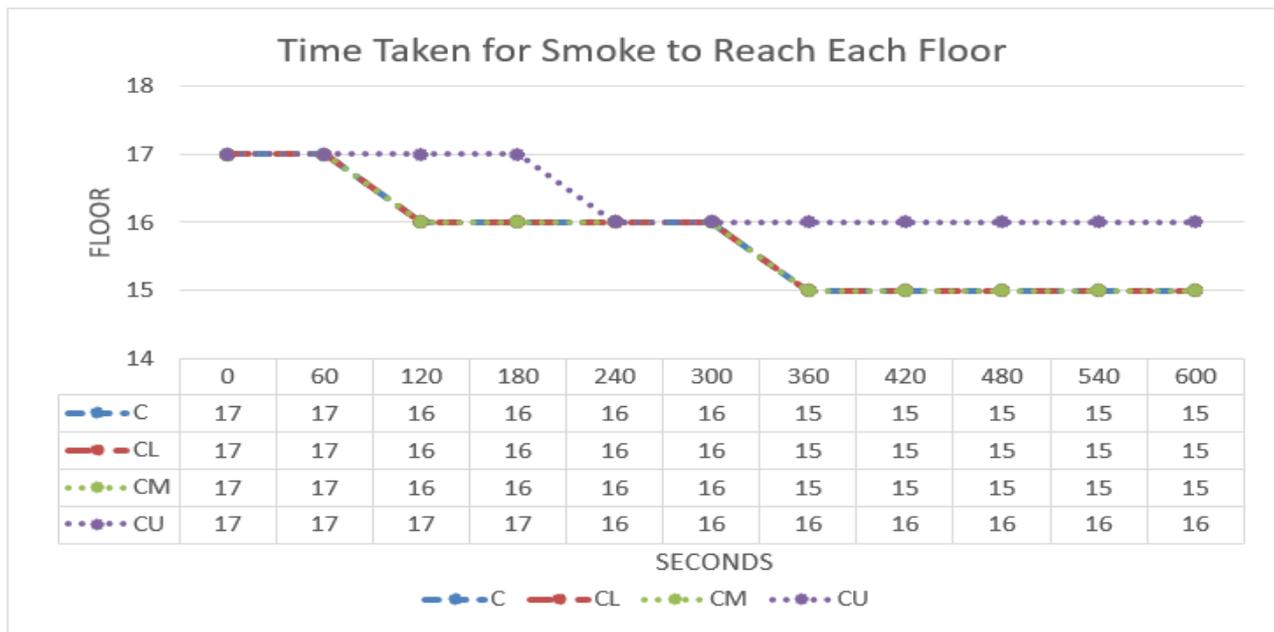
**Figure 7.** Time Taken for Smoke to Reach Each Floor in Case C,  $C_L$ ,  $C_M$  and  $C_U$ .
