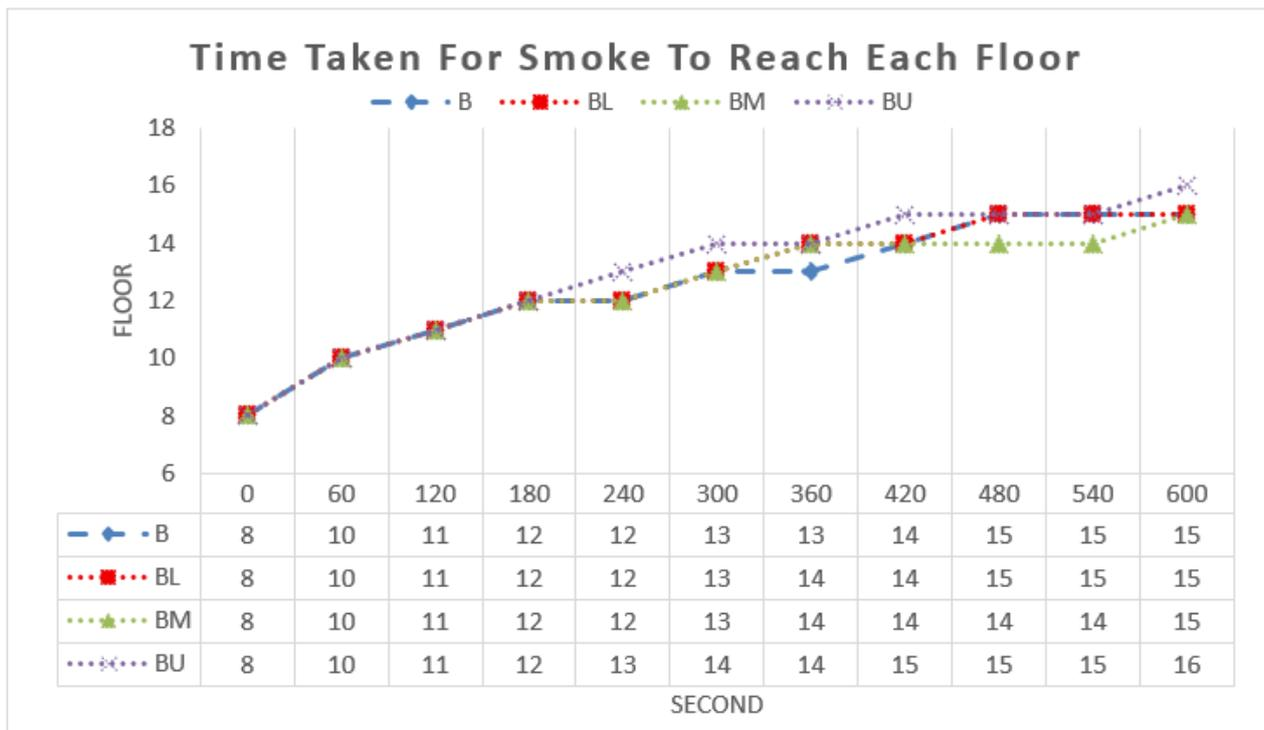
**Figure 6.** Time Taken for Smoke to Reach Each Floor in Case B, BL, BM and BU
