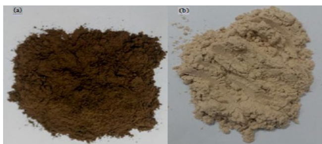
Figure 1. Post-processing images of (a) B. vulgaris lignin, and (b) B. vulgaris nanofiber.
