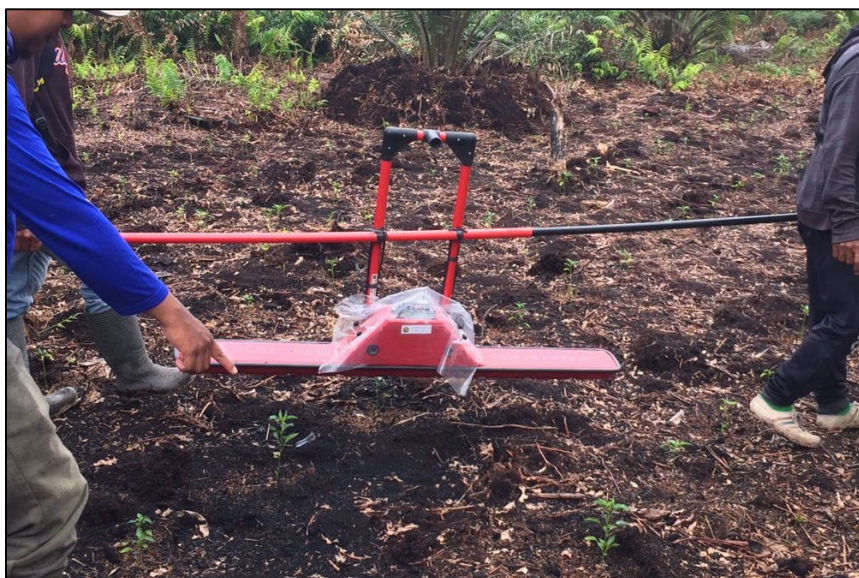
Figure 2. The GPR survey equipment, i.e., Plug-In Cobra GPR SE70
